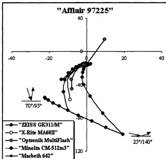
**Figure 9** / Comparison between the Measurement Data of Two Spectrophotometers With and Without Illumination Angle Variability
