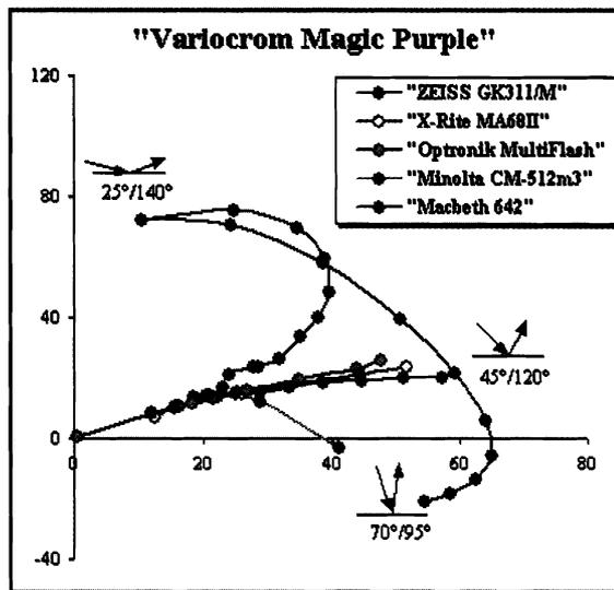
**Figure 13** / Comparison of Interference Shift under Various Illumination Angles and a Constant 15° Aspecular Angle and under Constant 45° Illumination and Various Cis-Trans Effect Angles
