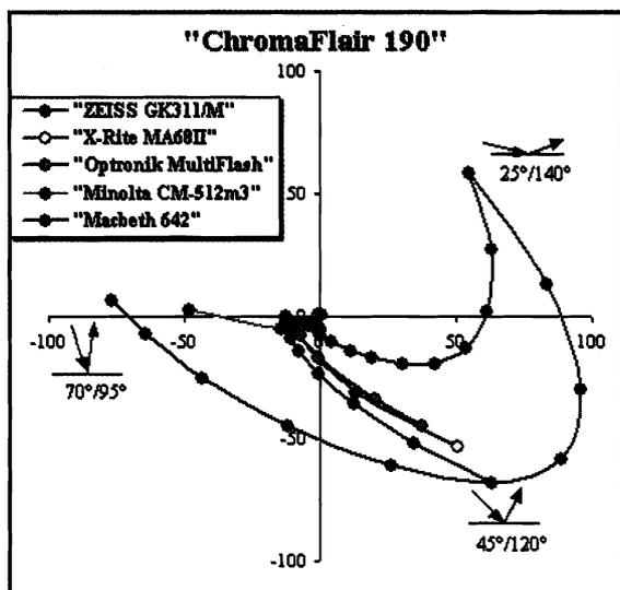
**Figure 12** / Interference and Aspecular Shift for a Liquid Crystal Effect Pigment in the a\*b\* Diagram of Various Measuring Instruments
