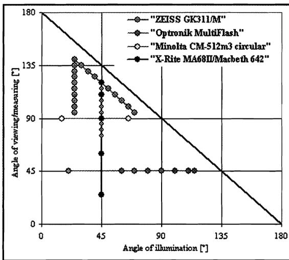
**Figure 7** / Schematic Comparison of the Geometries of Various Measuring Systems: The Zeiss GK 311/M Measures Under Constant Illumination or a Constant Aspecular Angle. The X-Rite and Macbeth Instruments Measure Under Constant Illumination; the Optronik MultiFlash Measures from a Constant Viewing Angle under Various Illumination Angles, the Effect Angle Being Cis or Trans to the Specular Angle
