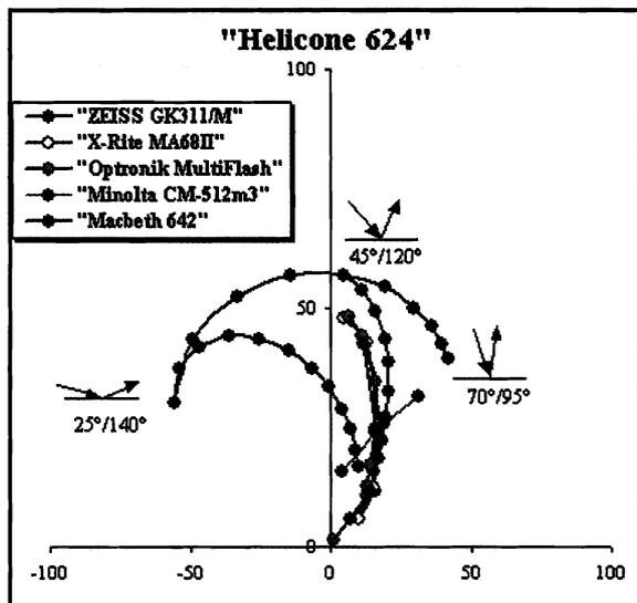
**Figure 11** / Interference and Aspecular Shift for a Multi-Layer Effect Pigment in the a\*b\* Diagram of Various Measuring Instruments
