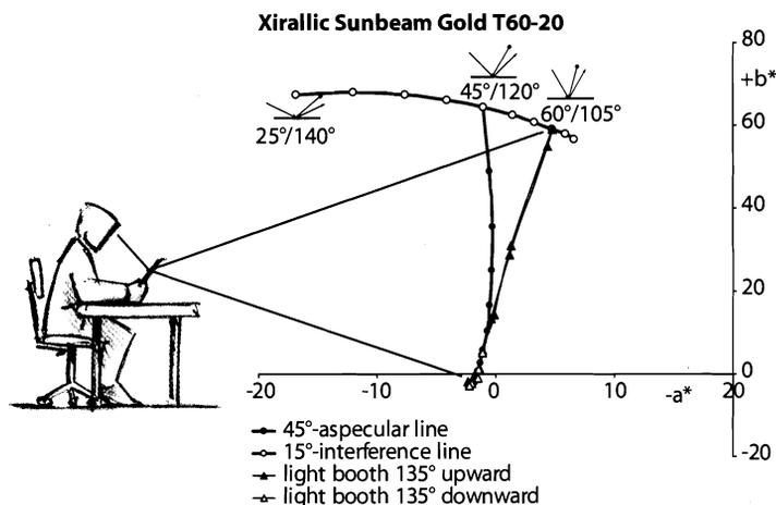
the arm involved outstretched and simultaneously walking toward the light source in order to allow the light source to illuminate the test panel at steeper angles of incidence. The important factor here is the parallel translation of the test panel necessary in order to maintain a constant difference between the angle of specular reflection and the viewing angle (Figure 8). The colors observed will then agree with instrumental characterizations.
