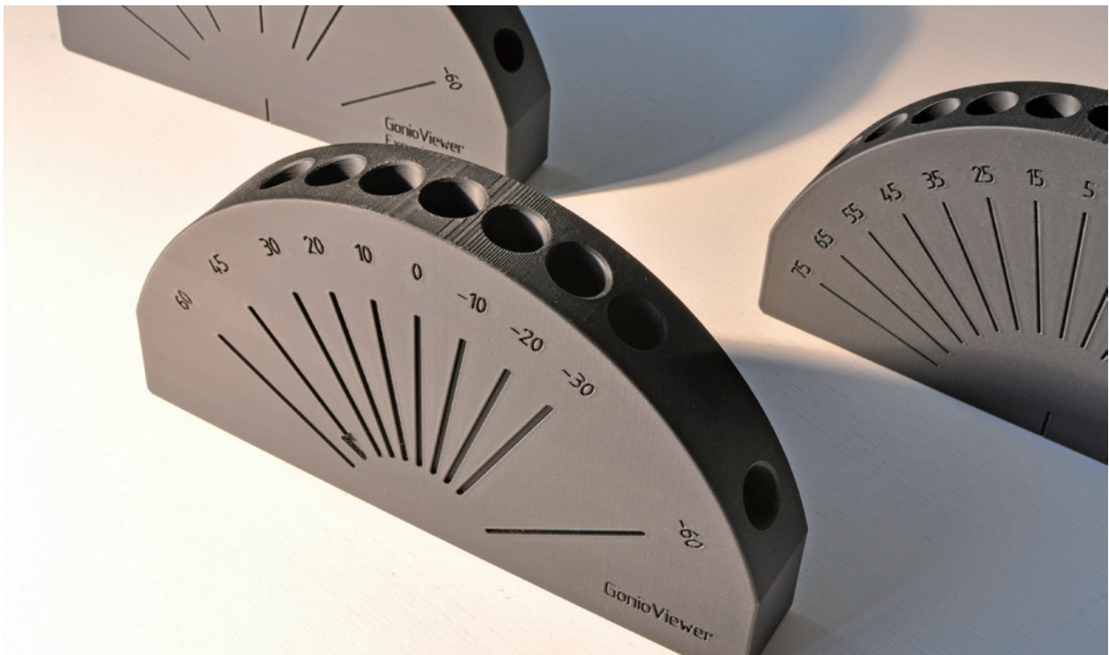
图1：GonioViewer 01具有与当前测量仪器相同的几何形状。额外的几何图形显示了新的干涉颜料的颜色梯度。 Figure 1: The GonioViewer 01 has the same geometries as the current measuring instruments. Additional geometries show the colour gradient of new interference pigments.
