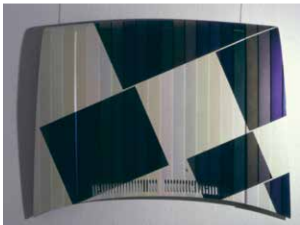
图1：车前盖板：先用白色涂布，然后表面用黑色涂布。从下到上，条纹已经被涂以不同的干涉色。根据视角，可以在白色底涂上识别出反射颜色或透射颜色。在黑色底涂上只有反射颜色可见。相应的透射颜色被黑色底涂吸收。 Figure 1: This bonnet has first been painted in white (Uni), From below to above, the stripes have been painted with different interference colours. Depending on the viewing angle, the reflection colours or transmission colours can be identified over the white undercoat. Over a black undercoat only the reflection colours are visible. The corresponding transmission colours are absorbed by the black undercoat.
